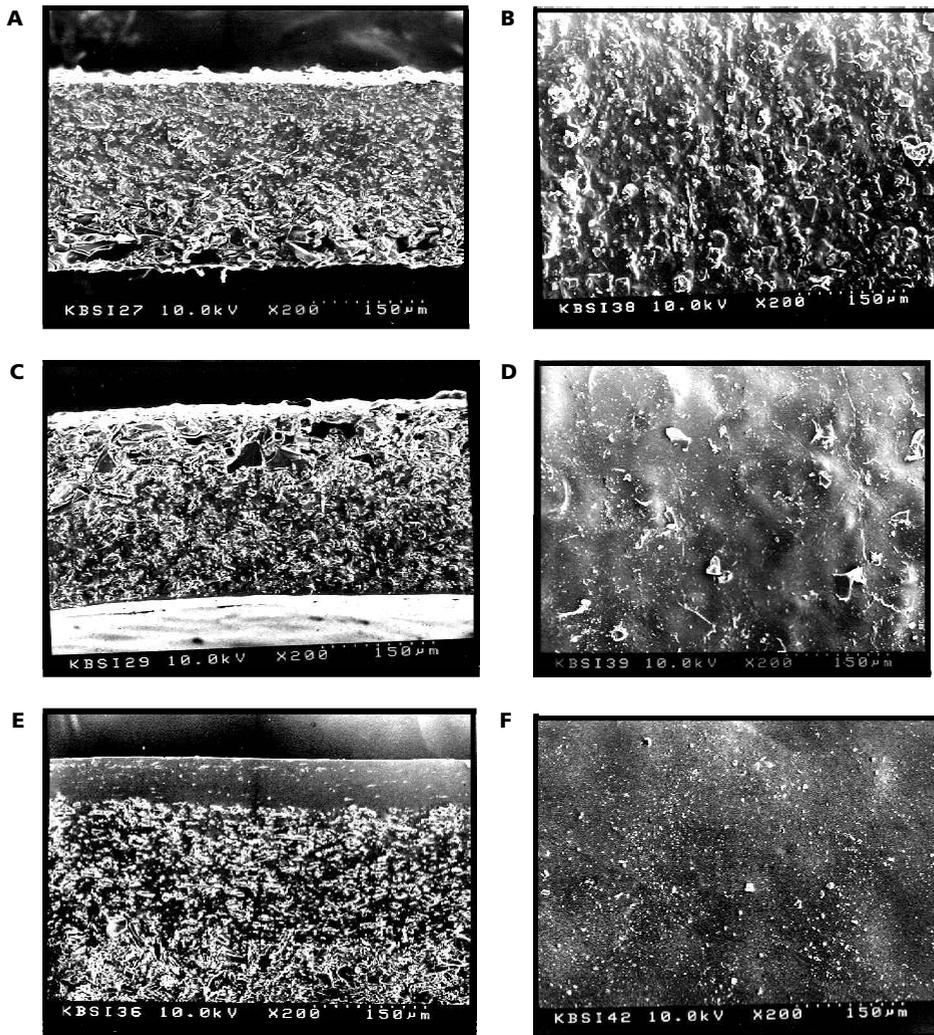
**Figure 2** SEM ( $\times 200$ ) of cross-section (A, C, E) and surface (B, D, F) of polyurethane matrices without coating (A, B) and after 3 coatings (C, D) or 10 coatings (E, F) produced by dipping in polyurethane–THF (1:40 w/w) solution. Each matrix contains 40% lyophilized powder (particle size, 62–88  $\mu\text{m}$ ; pore former–cefadroxil, 1:1), equivalent to 20% (w/w) pore former.
