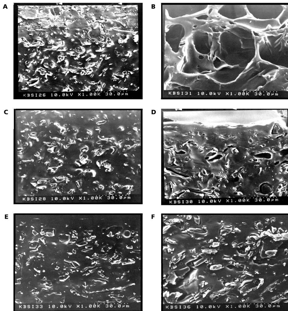
**Figure 3** SEM ( $\times 1000$ ) of cross-section of polyurethane matrices before (A, C, E) and after (B, D, F) in-vitro release study for 48 h. Each matrix contains 40% lyophilized powder (particle size, 62–88  $\mu\text{m}$ ; pore former–cefadroxil, 1:1) without coating (A, B) or with 3 coatings (C, D) or 10 coatings (E, F) produced by dipping in polyurethane–THF (1:40 w/w) solution.
